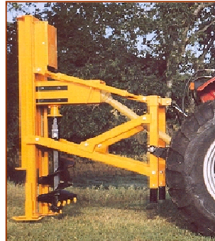
Rail Guided Drilling
