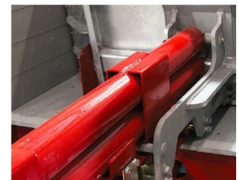
Simple, stacked push cylinders
