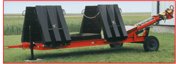
Driveover Pit, Transport
