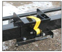
Header Brackets Adjust for Most Headers
