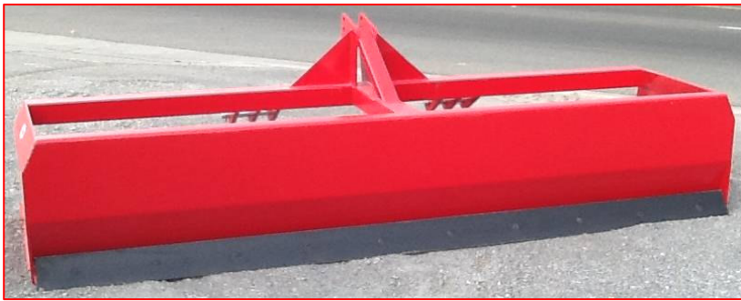
10' Scraper, Exclusive Reinforcing Bend and Skids on 3/8" End Plates, Cat 1-2 Hitch, Powder Coat Paint, Optional Rear Edge
